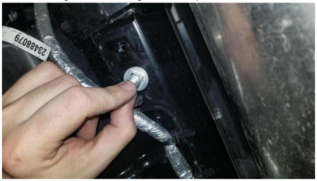
4. Grind out a 1" diameter hole. You need the bolt to pass through the frame. Use a step drill, or a grinding tool.
