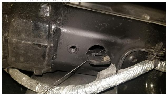
Pull the wire through the hole. This should pull the threads through the frame. 10.
