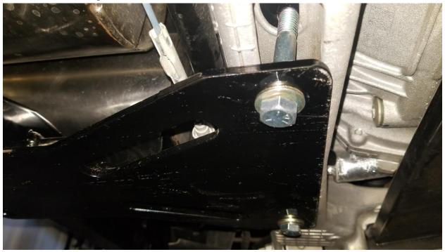
15. Center the hitch by measuring the distance to a fixed point on both sides of the vehicle.
