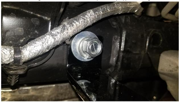
Put the mounting plate on top of the rear sub-frame. 13.
