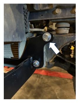
• Loosely thread two more 12mm bolts into the front lower threaded holes.
