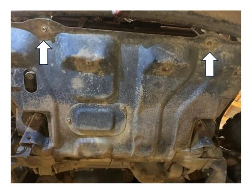
• Remove the two bottom screws fastening the factory brush guard to the vehicle frame and set the brush guard aside.
