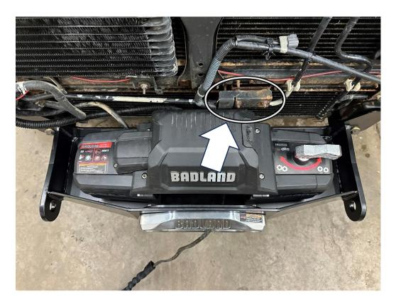
• \*\*\* Make sure winch or winch controller is not contacting the airbag sensor. Failure to complete this step can cause serious injury\*\*\*
