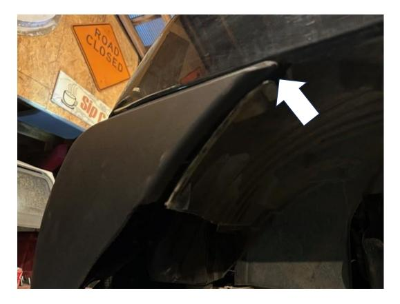
• Remove the bolts holding the factory front brush guard to the lower lip of the bumper cover.
