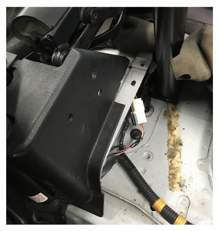
9. The panel mounts in with 4 bolts along the front bottom, and two on the top. The front bolt thread into the existing threaded holes that the parcel shelf used to use. The rear bolts require clip nuts as shown.
