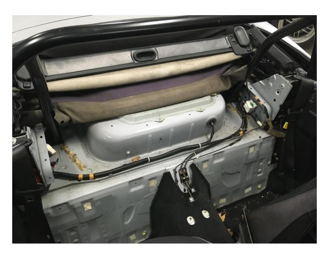
4. Install the 6 rubber grommets into the panel. A little water or WD-40 helps them slide in easier.
