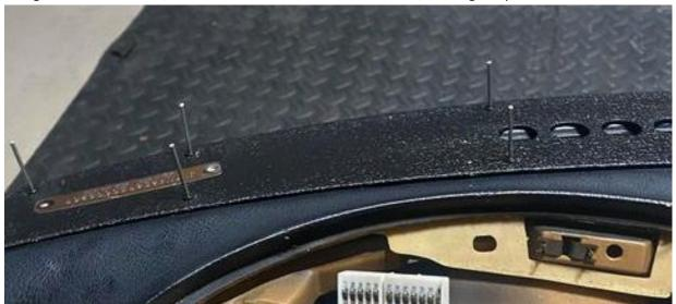
6. Reinstall the dash and enjoy! As an optional step, install a thin strip of foam on the leading edge of the dash before re-installing. This will keep the dash from rattling against the windshield.
