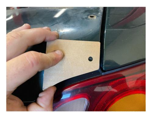
3. Pop out the two license plate lights. This will become the access hole for the retaining nuts on the center brackets.
