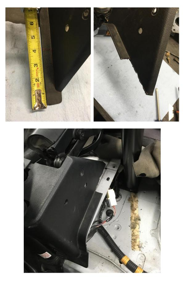
6. Run the 12V power supply wire from the battery to the amp location. Be sure to have the battery disconnected during this step. Mount the supplied fuse holder to the rear firewall behind the passenger seat. The amp will get mounted directly below this. It's a good idea to mock everything up and measure wire lengths before cutting.
