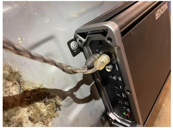
12. Install the panel into the car. Ensure the wires are run such that they reach the amp. Not the location in the picture below.
