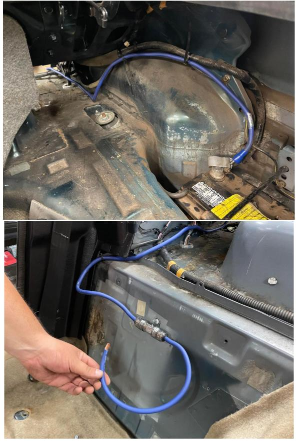
7. The Ground wire can be cut and mounted with the pre-existing 6mm threaded hole in the firewall as shown.
