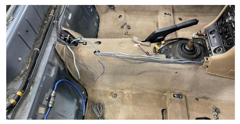
9. Next mount the amp using some self-tapping screws. We find it easiest to hold the amp in place, mark the hole locations and drill a pilot hole.
