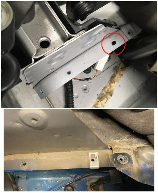
5. Before the panel is installed, you'll need to cut the lower ledge off the plastic trim pieces. A dremel or reciprocating saw works well. See pictures for where to cut. Once trimmed down, reinstall the panels.
