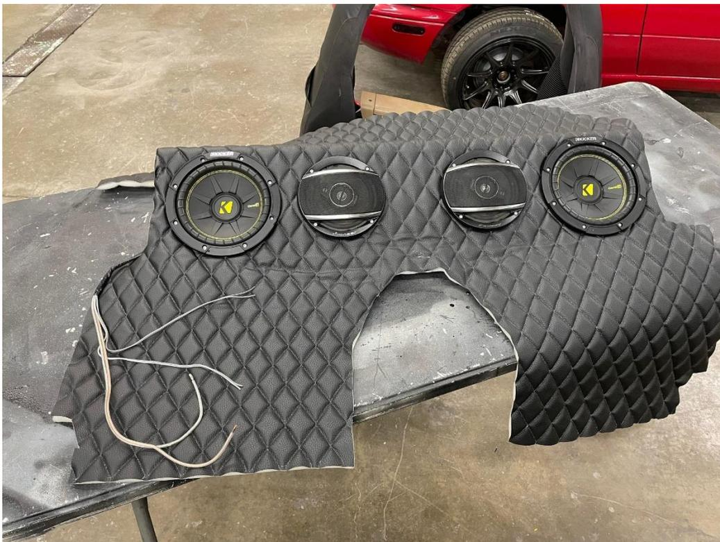
13. The panel is mounted with QTY 6 M6 screws with washers.
