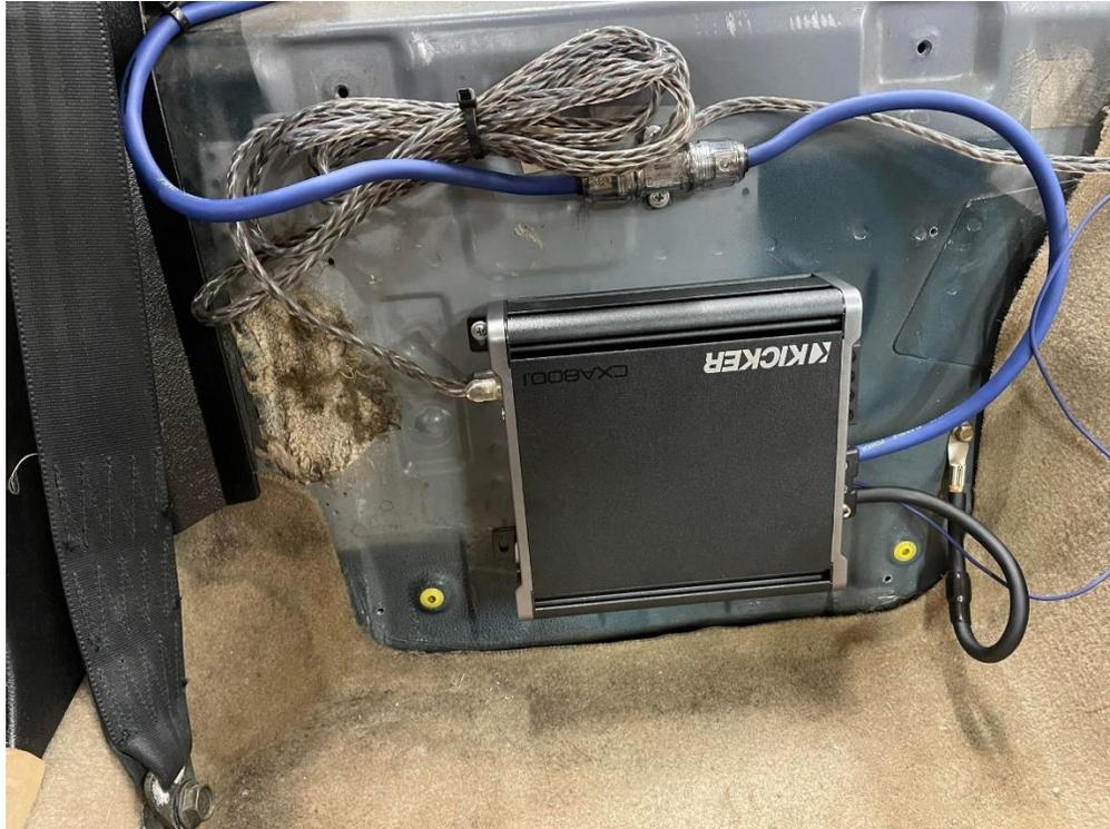
10. The power, ground and radio trigger wire are connected as shown.
