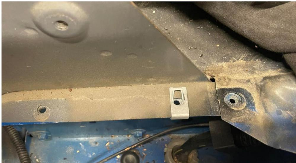
5. Before the panel is installed, you'll need to cut the lower ledge off the plastic trim pieces. A dremel or reciprocating saw works well. See pictures for where to cut. Once trimmed down, reinstall the panels.
