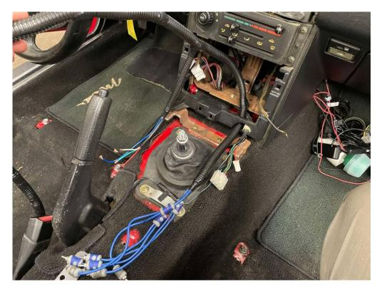
Once the harness is pulled through, connect the plug to the car's OEM harness.
