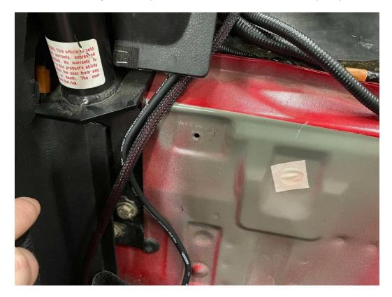
Position both the ground and power wires to the far left, under the B-pillar plastic.
