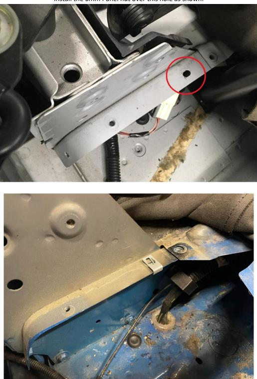
Install the 6mm Panel nut over this hole as shown.
