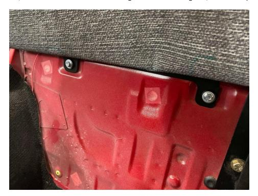
For 94-97 cars, install the LEFT two lower mounting screws. **DO NOT** tighten, install a couple of turns.
