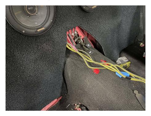
Route the speaker wires down the center of the car.
