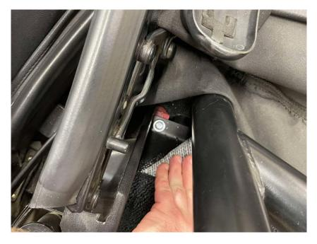
For 90-93, and 99-05 cars, install the RIGHT two lower mounting screws. **DO NOT** tighten, install a couple of turns.
