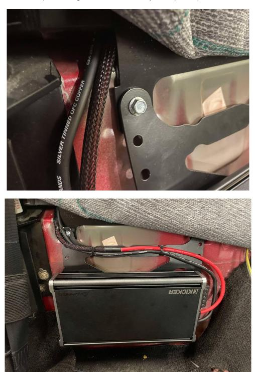
Route the power and ground cables to the amp, and zip-tie in place as shown.
