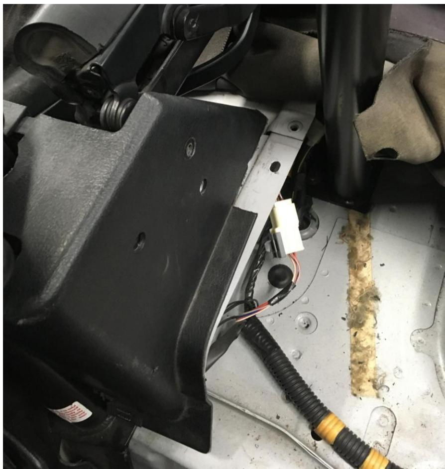
6. Run the 12V power supply wire from the battery to the amp location. Be sure to have the battery disconnected during this step. Mount the supplied fuse holder to the rear firewall behind the passenger seat. The amp will get mounted directly below this. It's a good idea to mock everything up and measure wire lengths before cutting.
