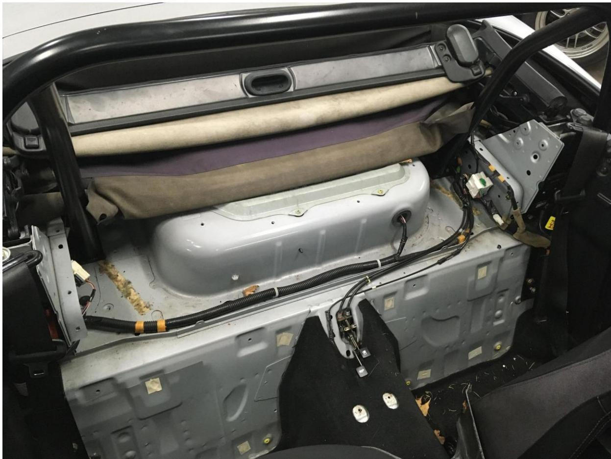
4. The panel mounts in with 4 bolts along the front bottom, and two on the top. The front bolt thread into the existing threaded holes that the parcel shelf used to use. The rear bolts require clip nuts as shown.
