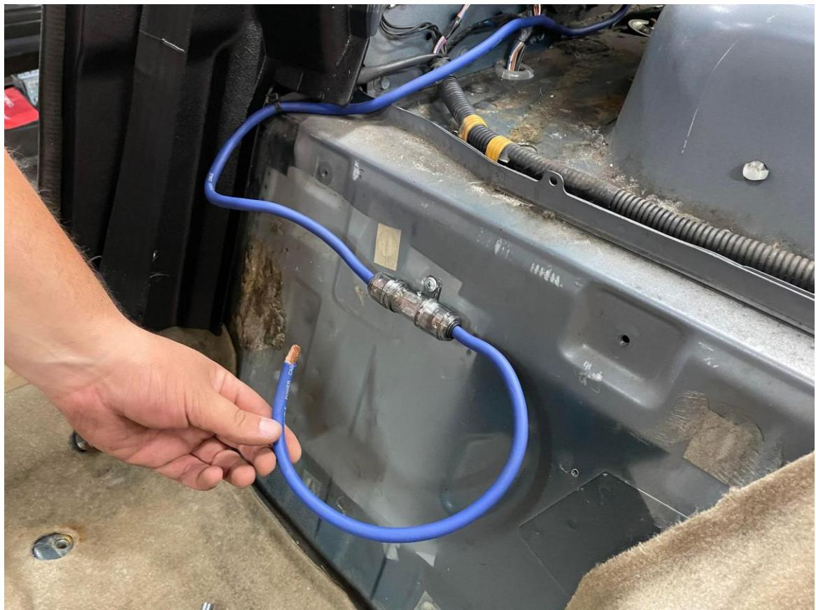
7. The Ground wire can be cut and mounted with the pre-existing 6mm threaded hole in the firewall as shown.
